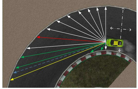
Fig. 2: The red vector, the yellow vector, green vectors, and the blue vector represent the zero sensor, the base sensor, auxiliary sensors, and the final angle to take the turn, respectively.
