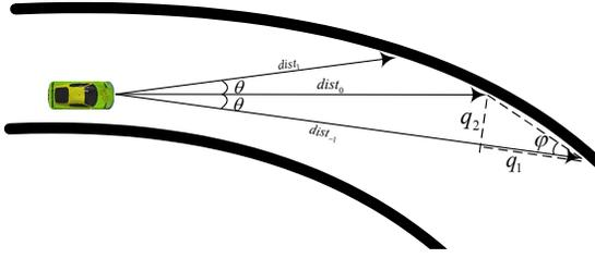
Fig. 1: The angle of the turn in front is estimated based on  $dist_{-1,0,1}$  sensors.
