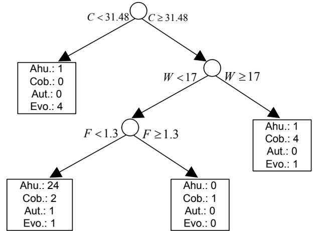
Fig. 13: Decision tree for classification of controllers on different tracks in the race stage. W is the width of the track. The results are the average number of standing first over 5 runs.
