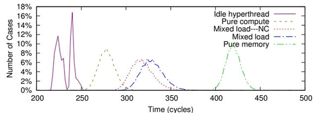
Fig. 4 Distribution of time to write 32 entries at an offset on a Skylake Processor.
