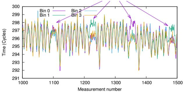
Fig. 7 Measurement trace of OpenSSL RSA decryption—detailed view
