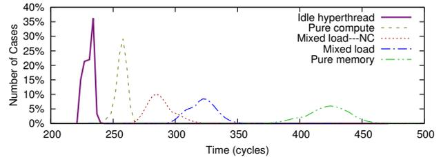
Fig. 3 Distribution of time to read 256 entries from a cache bank on a Sandy Bridge Processor.
