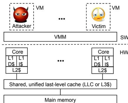
Fig. 1: System model for a multi-core processor
