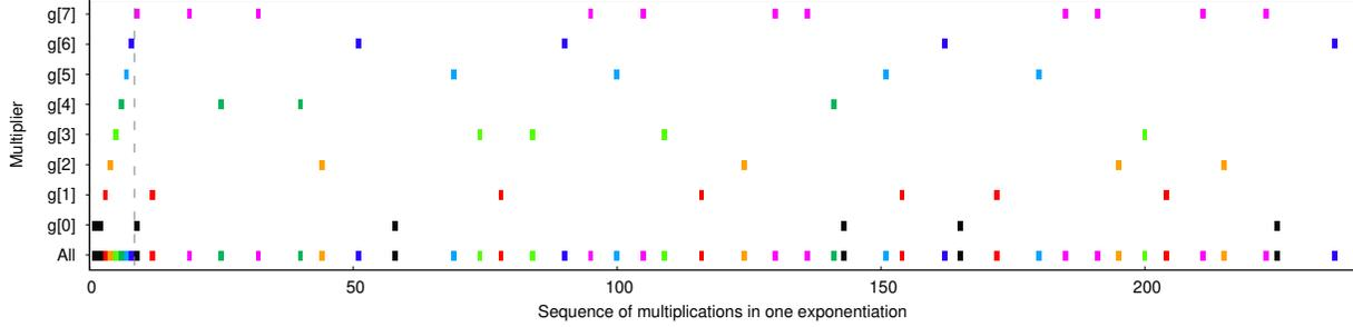
Fig. 8: The usage patterns of the multipliers  $g[i] = b^{2^{i+1}}$  in an exponentiation. The vertical line separates the pre-computation and the body of the exponentiation. The x-axis shows the first 240 of 492 multiplications in the exponentiation.
