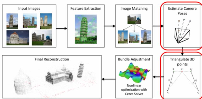
The  $L_\infty$  formulation can solve core subproblems in the Structure-from-Motion (SfM) pipeline.
