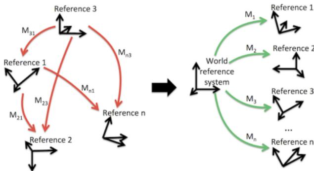
Determine absolute camera rotations from pairwise relative measurements.
