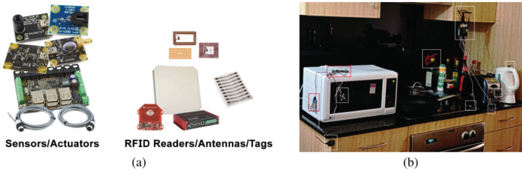
Fig. 5. The settings of system: (a) some sensors and RFID devices, and (b) part of the kitchen setting (e.g., sensor-enabled microwave oven and toaster).
