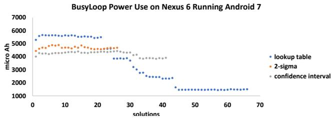
Fig. 5: Solution fitness values of busy loop optimisation experiment. The measurements are the ones returned by the internal meter for the solutions shown in Figure 4 and thus exhibit a slight upwards trend due to sensor drift.
