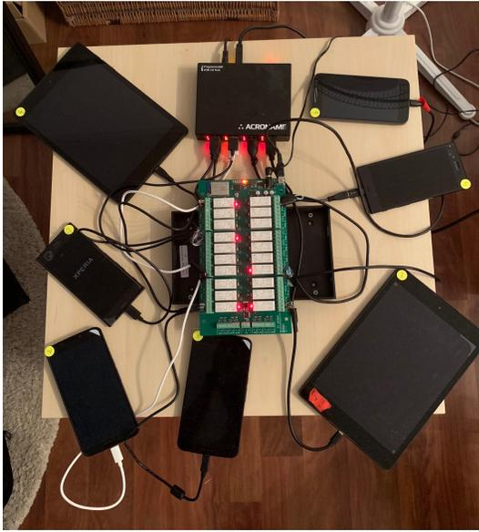
Fig. 2: Phone farm in action, multiple experiments running in parallel. The relay in the centre is responsible for physically disconnecting the phones from the charger. Screens are off to minimise noise from the screen’s consumption, and wake-locks are used to prevent the from entering various standby modes.
