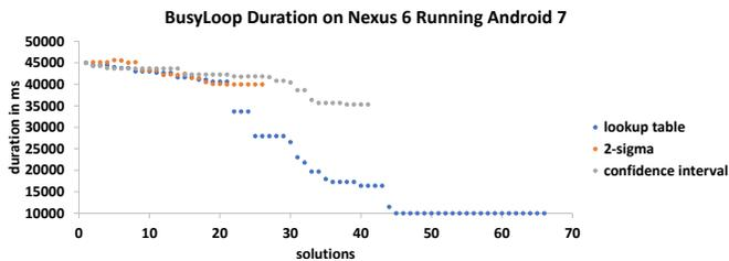
Fig. 4: Solutions’ duration of busy loop optimisation experiment, shown are tournament winners. The duration equals the value of the decision variable.
