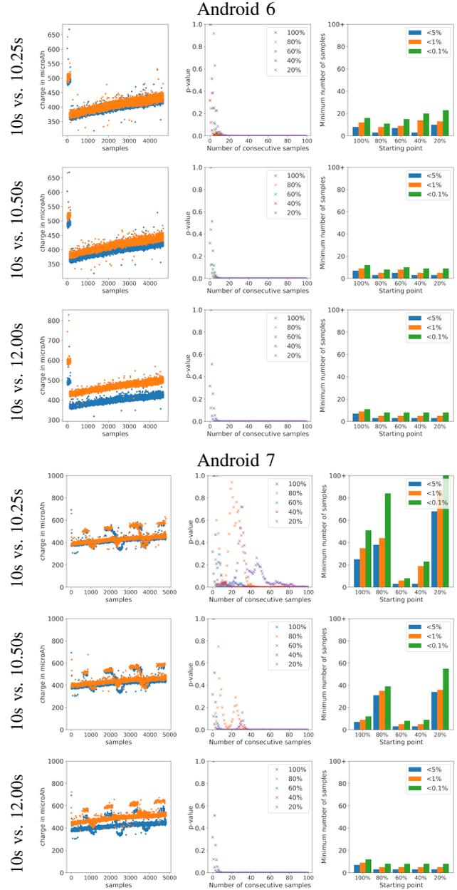
Fig. 3: Power use of repeated runs of BusyLoop app on Moto G4 Play. Blue: 10s, orange: as listed.
