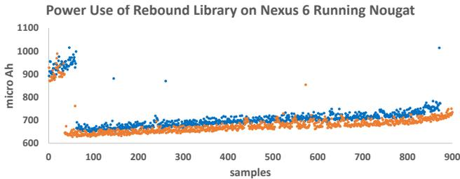
Fig. 1: Power use of repeated runs (“samples”) of the original Rebound library on Nexus 6 running Android 7. Setup: Rebound was run 900 times (blue), then the device was recharged, then Rebound was run again 900 time.
