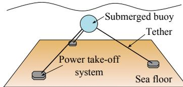
Fig. 1: Schematic representation of a three-tether WEC [24].
