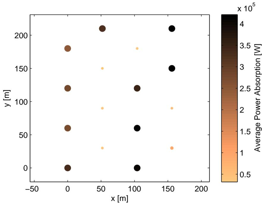
Figure 4.7: The radii configuration of the best RCW-based solution found by RLS for the 4x4 array. RCW = 0.920; q-factor = 0.853; Power = 3,751,603; Tether Force = 590,251.
