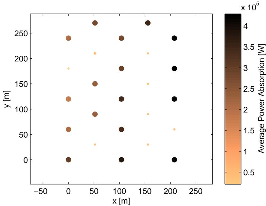
Figure 4.9: The radii configuration of the best RCW-based solution found by RLS for the 5x5 array. RCW = 0.839; q-factor = 0776; Power = 5,622,107; Tether Force = 592,966.
