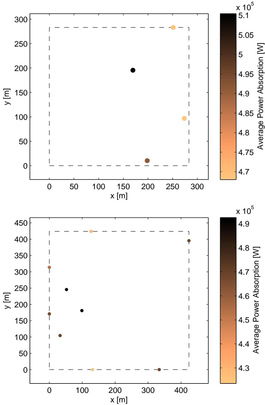
Figure 6.3: The best layouts found for the 2x2 and 3x3 arrays when optimising for RCW. The optimisation criteria values of these layouts are given in Table 6.2.
