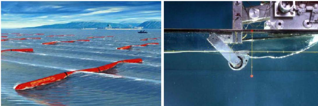
Figure 2.1: Examples of attenuator (left) and terminator (right) WECs [13].
