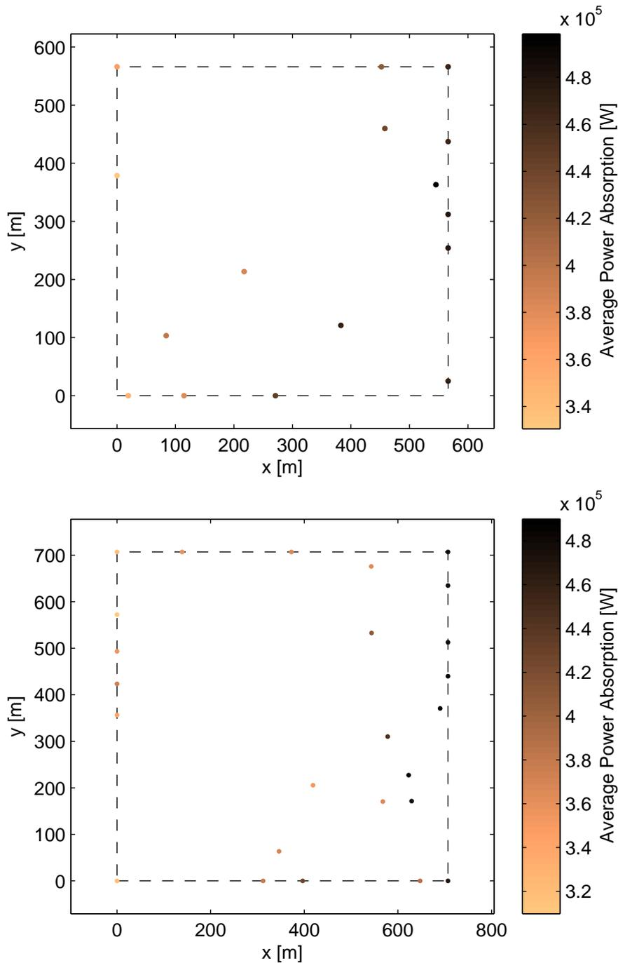
Figure 6.7: The best layouts found for the 4x4 and 5x5 arrays when optimising for q-factor. The optimisation criteria values of these layouts are given in Table 6.3.
