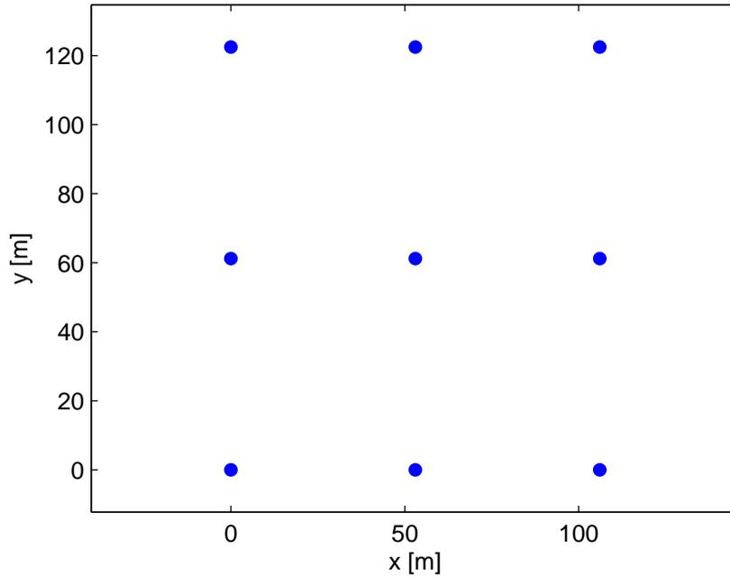
Figure 5.1: The aligned grid layout of a 3x3 array in the CETO model.
