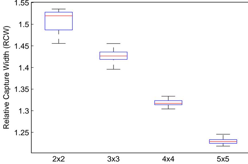
Figure 6.2: The RCW of the best solutions found in each repetition of CMA-ES layout optimisation. The results are grouped by array size.
