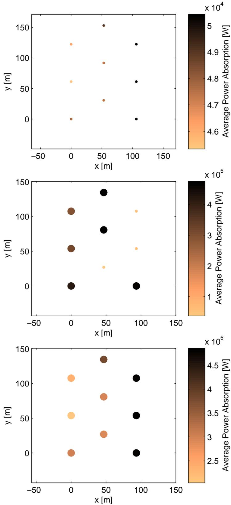
Figure 4.5: The optimal radii configurations of the 3x3 array. The top configuration is optimal for q-factor and tether force, the middle configuration is optimal for RCW, while the bottom configuration is optimal for average power absorption.
