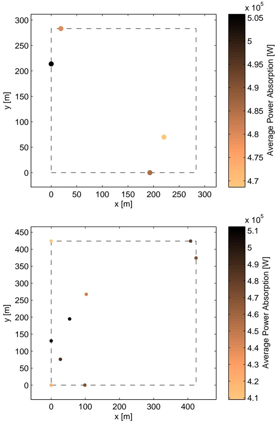
Figure 6.6: The best layouts found for the 2x2 and 3x3 arrays when optimising for q-factor. The optimisation criteria values of these layouts are given in Table 6.3.
