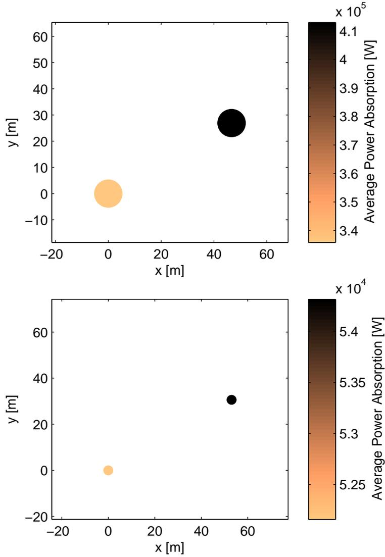
Figure 4.3: The optimal radii configurations of the 2x1 array. The top configuration is optimal in terms of RCW and average power absorption. The bottom configuration is optimal in terms of q-factor and tether force. The direction of wave propagation is from right to left.
