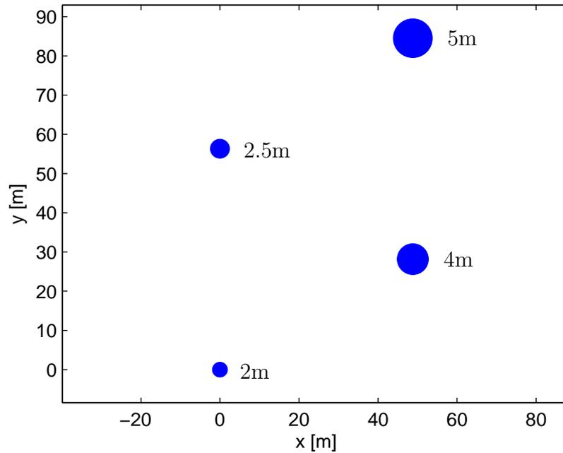
Figure 4.1: The  $(2 \ 2.5 \ 4 \ 5)$  radii configuration of a 2x2 array using a staggered layout. The direction of wave propagation is from right to left.
