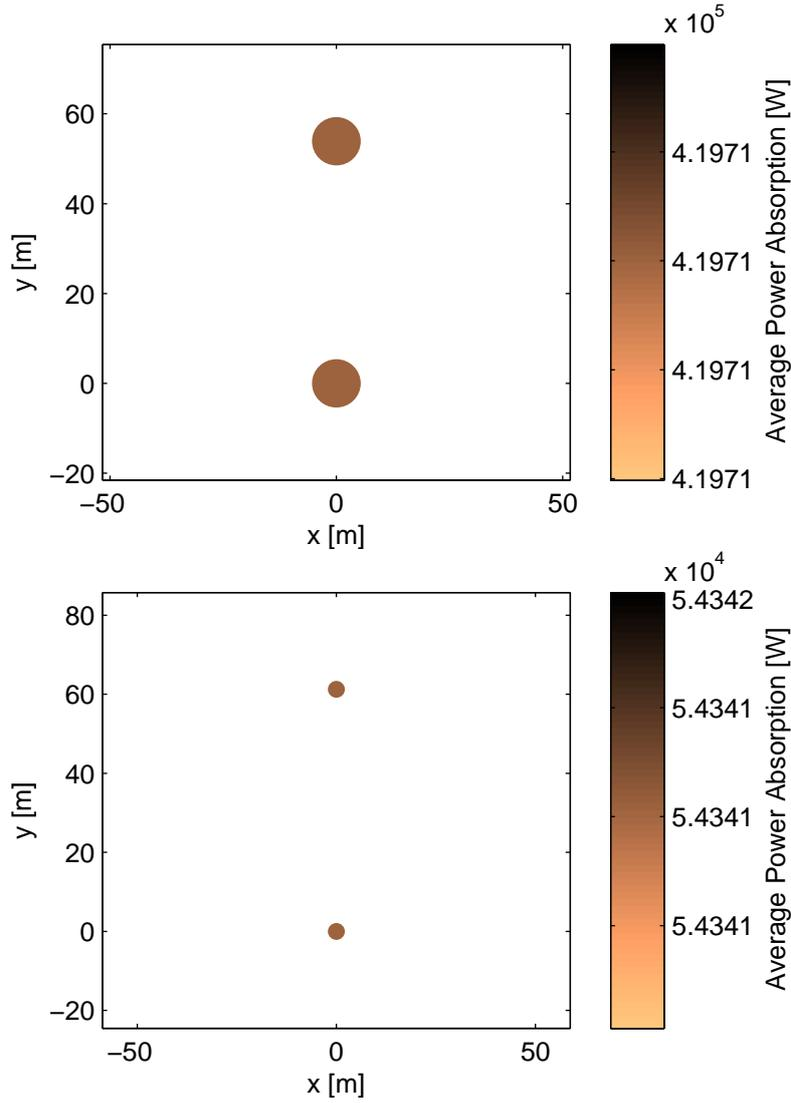
Figure 4.2: The optimal radii configurations of the 1x2 array. The top configuration is optimal in terms of q-factor, RCW and average power absorption. The bottom configuration is optimal in terms of tether force.
