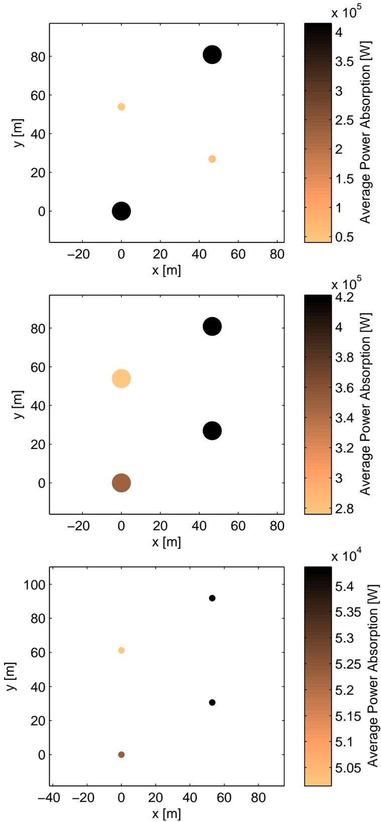
Figure 4.4: The optimal radii configurations of the 2x2 array. The top configuration is optimal for q-factor, the middle configuration is optimal for RCW and average power absorption, while the bottom configuration is optimal for tether force.
