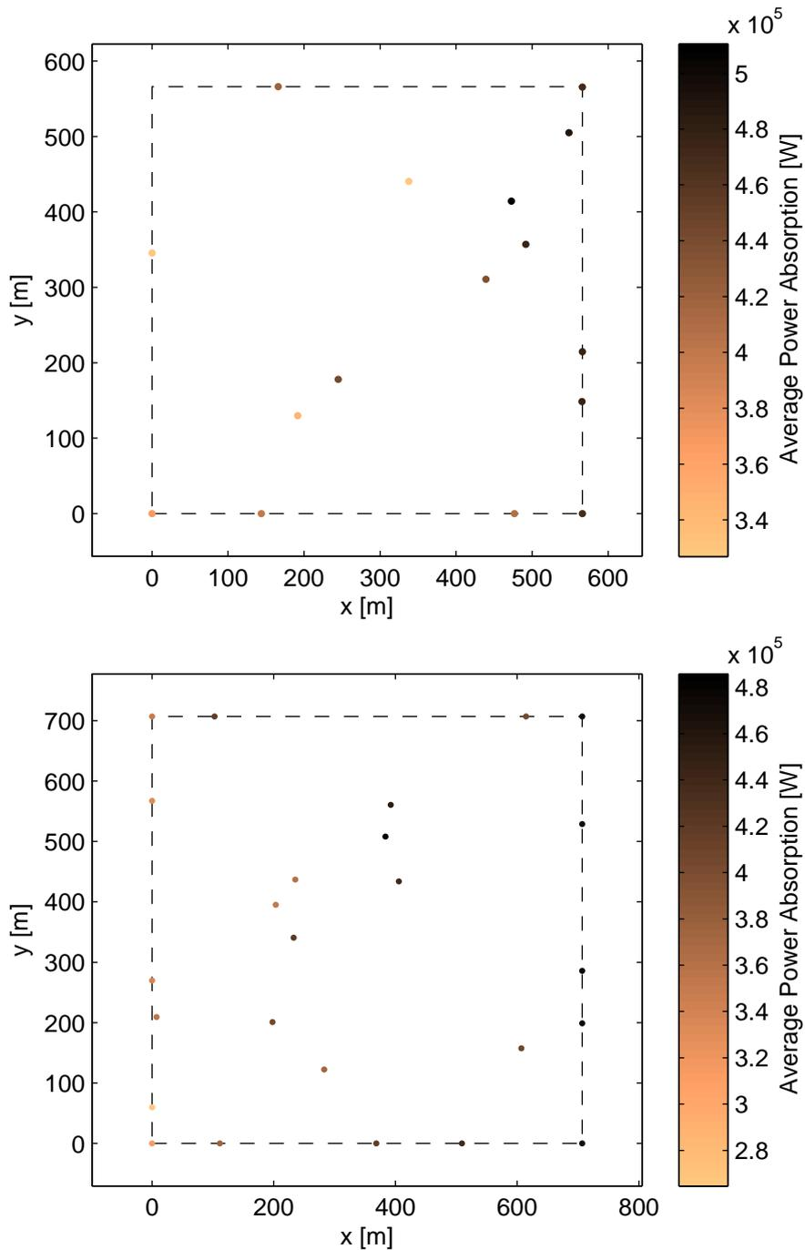
Figure 6.4: The best layouts found for the 4x4 and 5x5 arrays when optimising for RCW. The optimisation criteria values of these layouts are given in Table 6.2.
