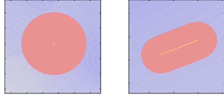
Fig. 3. One building (gray) and one street (yellow) surrounded by constrained red areas. In the background the structure of the wind potential at position is shown.
