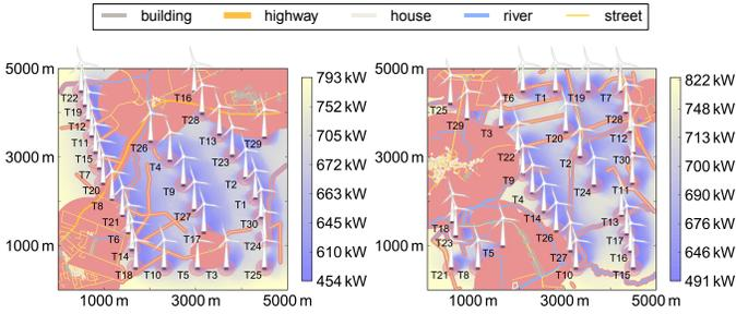
Fig. 8. Left: best solution for Scenario 1 with balanced penalty function using  $G_{[G_N \in \mathbb{R}]}$  and random initial solution, right: best solution for Scenario 2 with balanced penalty function using  $G_{[N_t \in \mathbb{R}]}$  and feasible initialization
