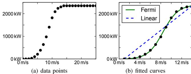
Fig. 1. Power curve of wind turbine E92
