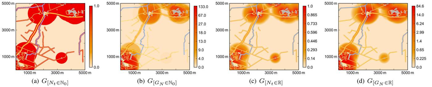
Fig. 5. The induced penalty  $G$  when placing one turbine on the map in Scenario 1 for the penalty variants  $G_{[N_t \in \mathbb{N}_0]}$ ,  $G_{[G_N \in \mathbb{N}_0]}$ ,  $G_{[N_t \in \mathbb{R}]}$ , and  $G_{[G_N \in \mathbb{R}]}$ . The non-linear colorbars with different scalings illustrate the resulting penalty functions  $G$ .
