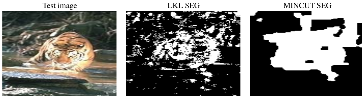
Figure 3. Water detection results. Dark area represents regions of the image containing the concept water.
