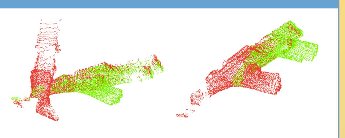
**Comparison against RANSAC.** Transforms were estimated by three keypoint matches and the quality was taken over all the points. We stopped RANSAC as soon as  $Q_{qlob}$  equalled or surpassed the  $Q_{alob}$  of the BnB methods, or if the number of iterations hit the limit of 50000. The median results from 20 instances of RANSAC are reported.
