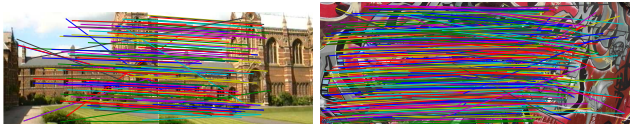
Figure 4. SIFT keypoint matches on two image pairs: Keble (left) and Graf (right), for Homography estimation in Sec. 5.1.
