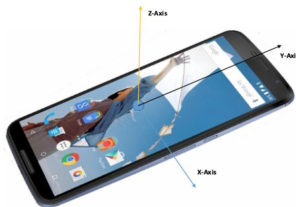
Figure 2.1: Axis Position on Phone
