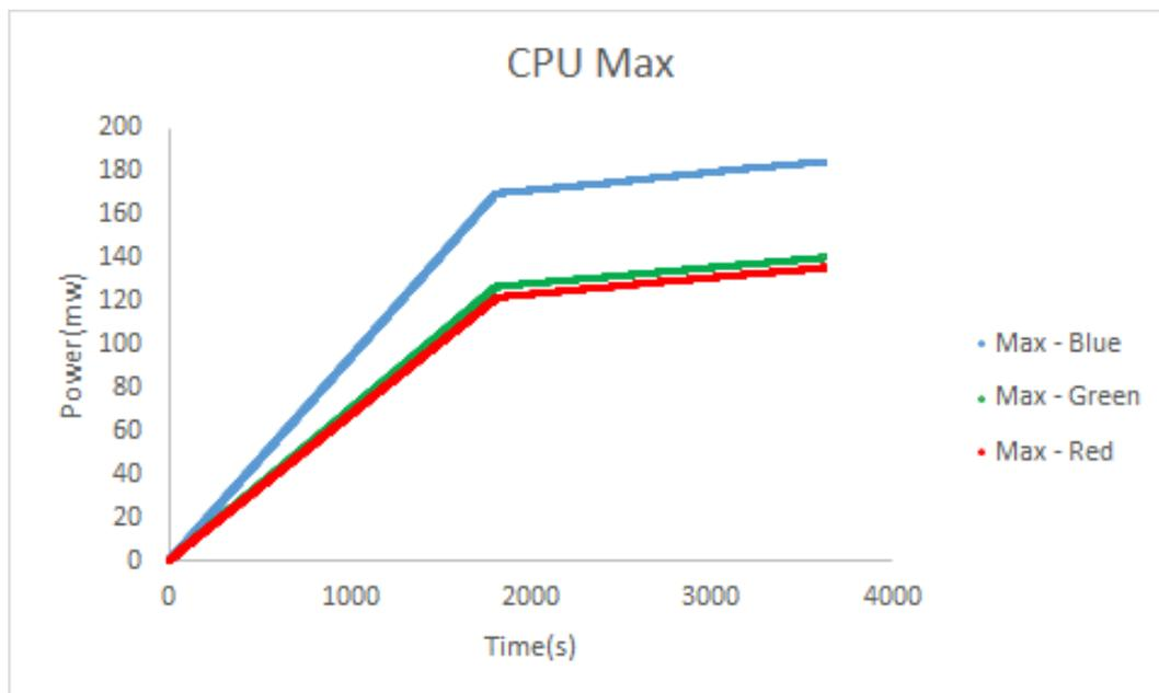
Figure 4.5. Total Power consumption for different color in max CPU Frequency
