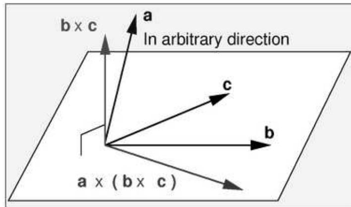
$$\begin{aligned}(\mathbf{a} \times (\mathbf{b} \times \mathbf{c}))_1 &= a_2(\mathbf{b} \times \mathbf{c})_3 - a_3(\mathbf{b} \times \mathbf{c})_2 \\&= a_2(b_1c_2 - b_2c_1) + a_3(b_1c_3 - b_3c_1) \\&= (a_2c_2 + a_3c_3)b_1 - (a_2b_2 + a_3b_3)c_1 \\&= (a_1c_1 + a_2c_2 + a_3c_3)b_1 - (a_1b_1 + a_2b_2 + a_3b_3)c_1 \\&= (\mathbf{a} \cdot \mathbf{c})b_1 - (\mathbf{a} \cdot \mathbf{b})c_1\end{aligned}$$
