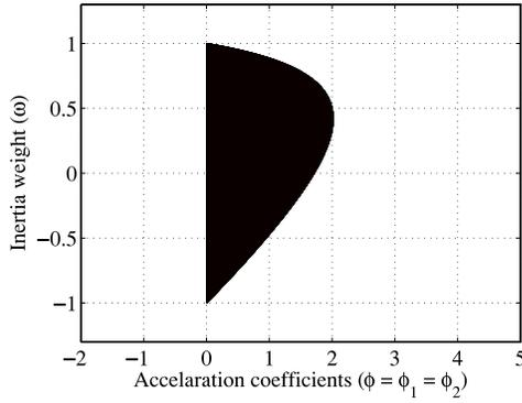
Fig. 1. Convergence boundaries for IPSO (dark area) that were reported in [24] through theoretical analysis.
