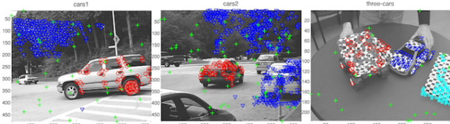
Figure 6. The “cars1”, “cars2”, and “three-cars” data with 10% gross outliers (marked as “+”) for fundamental matrix estimation.
