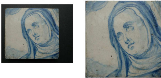
Fig. 5. Tile acquisition and correction. Left: tile acquired by a camera. Right: corrected tile, considering perspective and size. Image provided by Fonseca [5].
