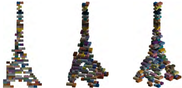
Figure 18. Three views of the reconstruction achieved using the images from Figure 16, without support constraints. The optimization in this case took less than 2 minutes, but has many holes and unsupported blocks.
