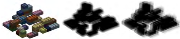
Figure 5. A synthetically generated test scene, and two images showing the magnitude of the noise added to the synthetic image formation process. The images were generated by adding together 10 silhouettes of the scene, each of which had noise of 0.3 or 0.5 (respectively) added to the camera parameters.
