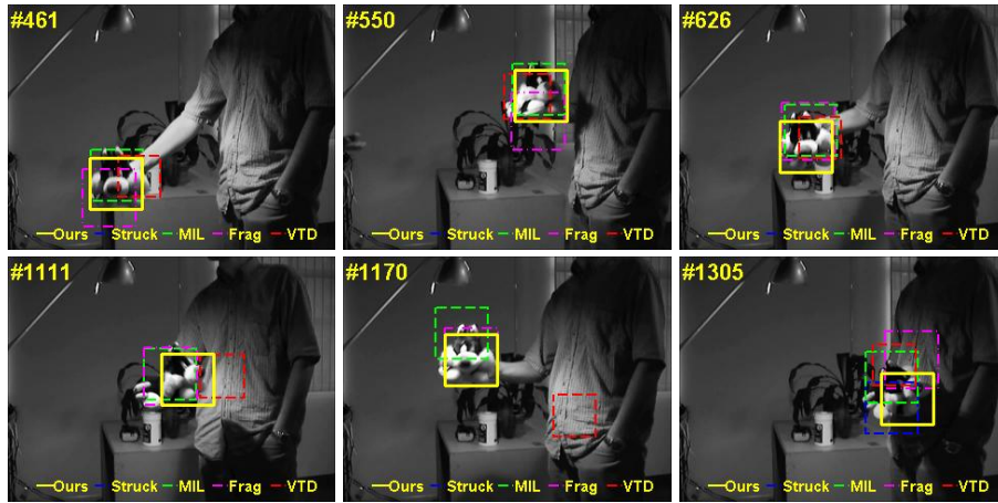
Fig. 10. Sequence sylv : The tracking results of different tracking approaches over representative frames.
